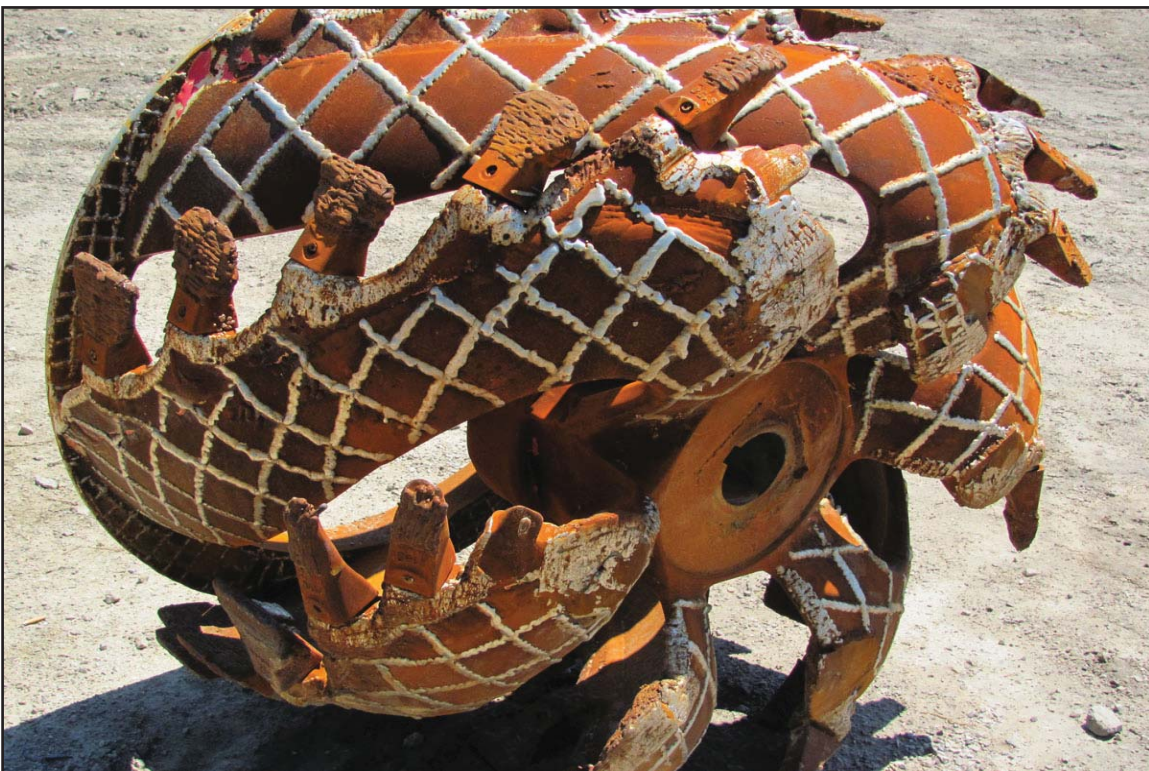
2H - Severson 20-inch cutter head with hard facing and teeth for hard dredging. May 5, 2010.
