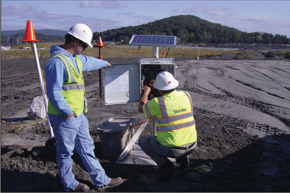
9G - Monitoring of piezometer instrumentation. September 30, 2009.
