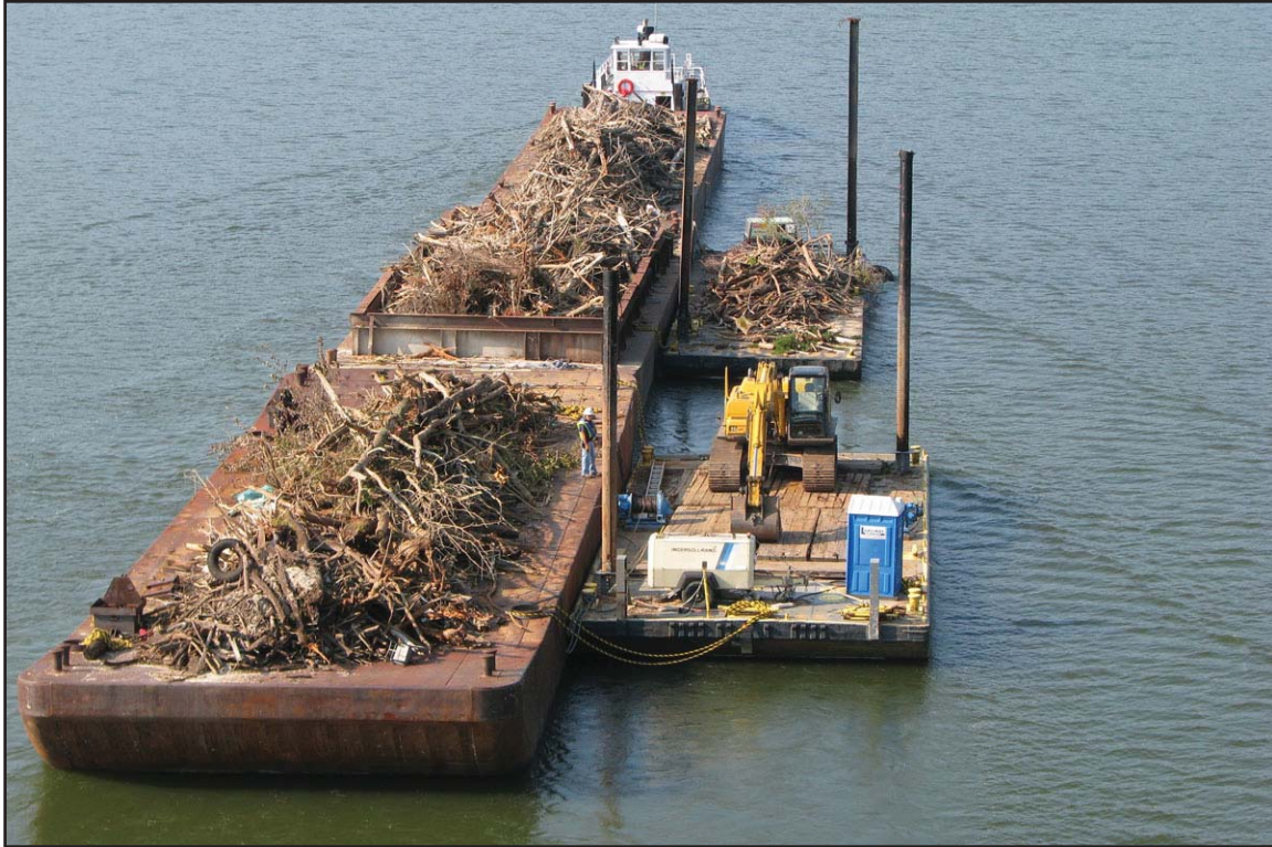
7I - Debris barge used to transport debris back to the Kingston Fossil Plant. August 24, 2009.
