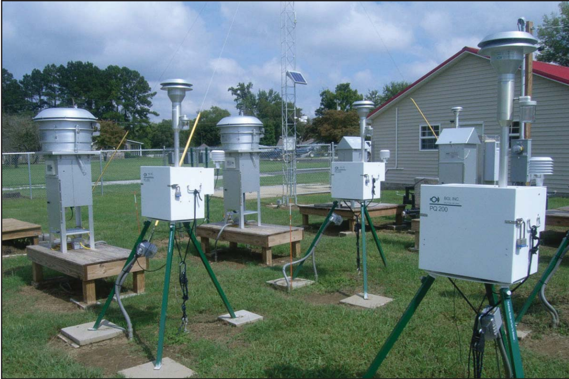
10I - Air monitoring equipment used to measure dust particulate and metal concentrations in air around the site. September 22, 2009.
