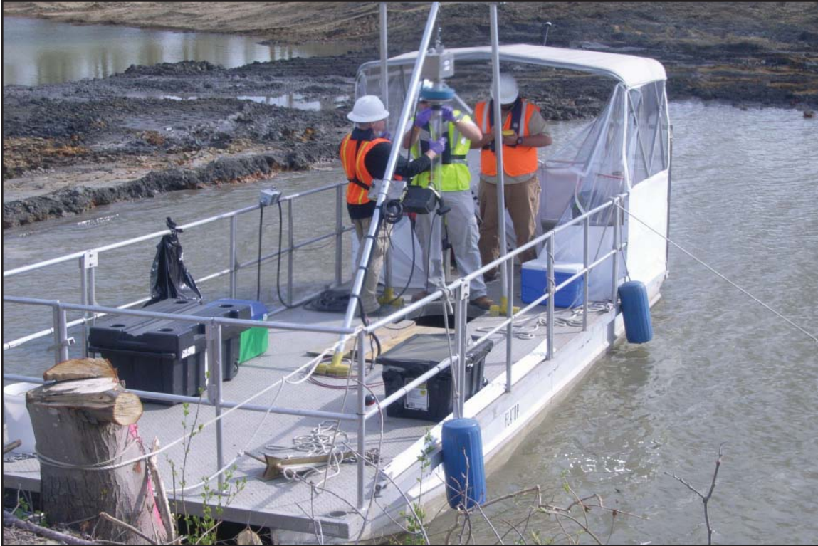
2Y - Vibecore sampling boat and equipment used to collect sediment samples to confirm ash removal. April 7, 2010.
