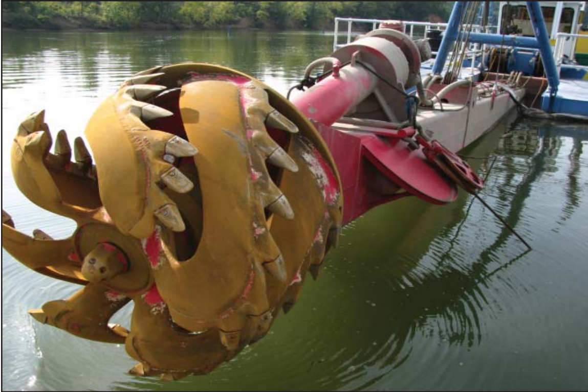
2I - Severson 16-inch cutter head and boom for deeper cut. September 1, 2009.
