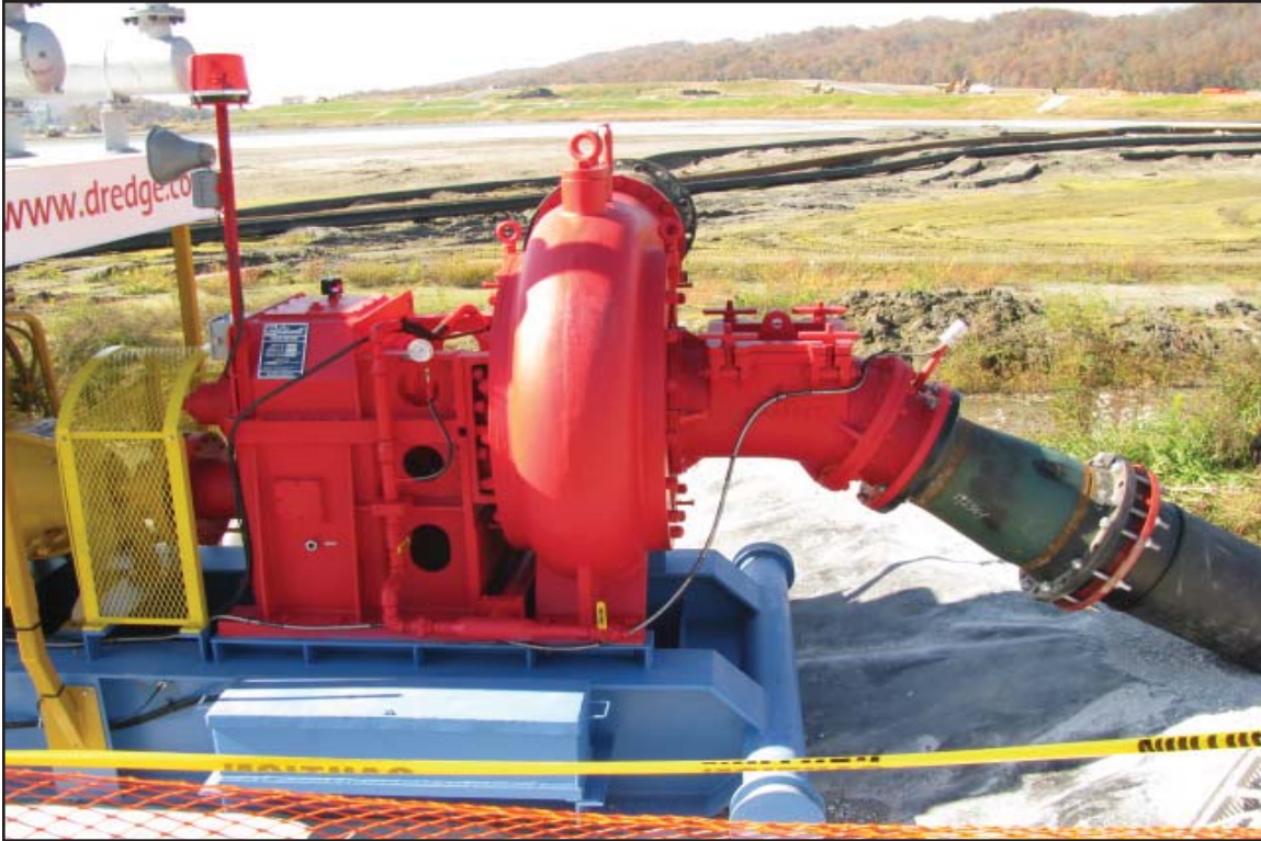
20 - Dredge discharge line booster pump. November 7, 2009.
