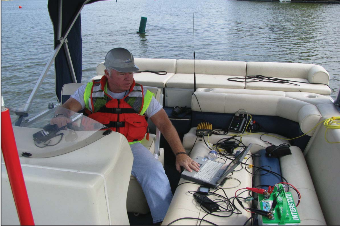
2W - Bathymetric survey boat and equipment used to measure elevation of river bottom. October 29, 2009.
