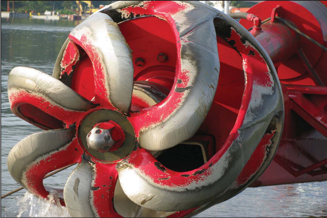
2G - Severson 14-inch dredge cutter head showing wear due to dredging. August 1, 2009.
