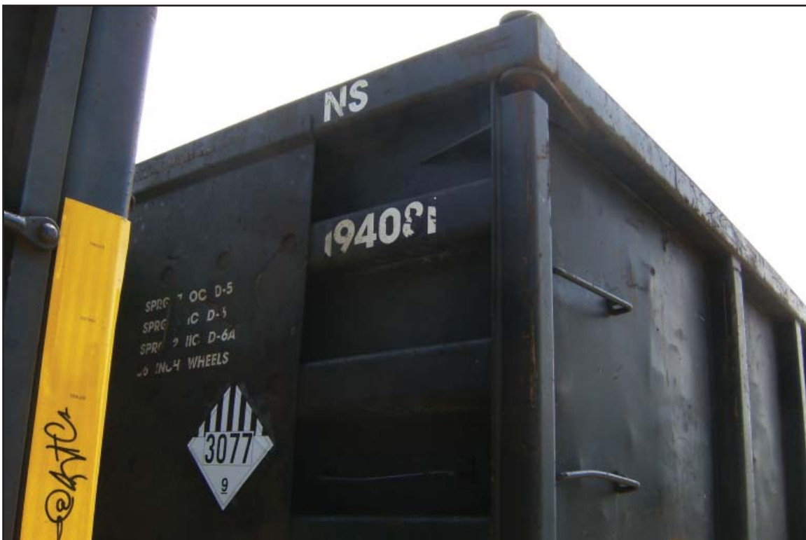
6L - Typical ash disposal railcar placarding.
