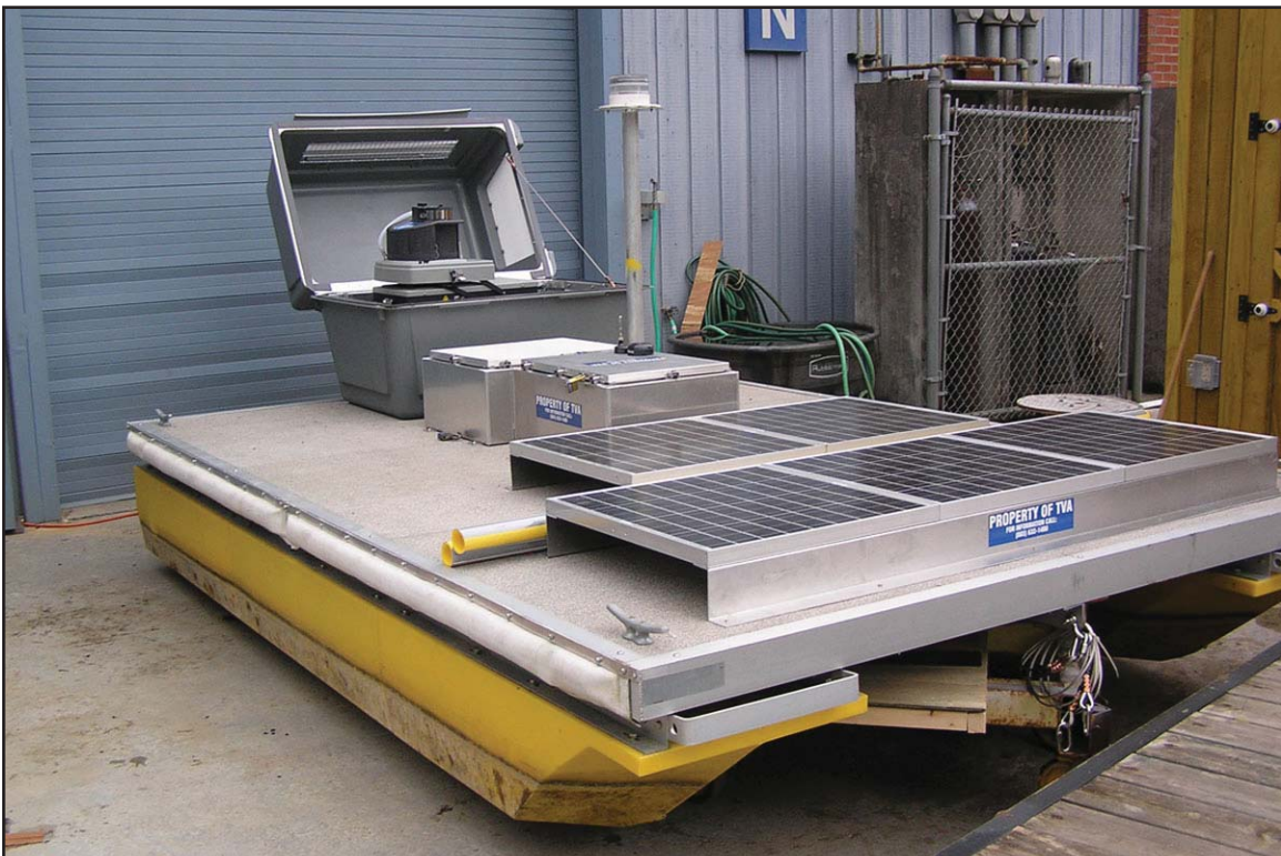
10L - Hydrolab equipment used to collect surface water samples in Watts Bar Reservoir. December 15, 2009.
